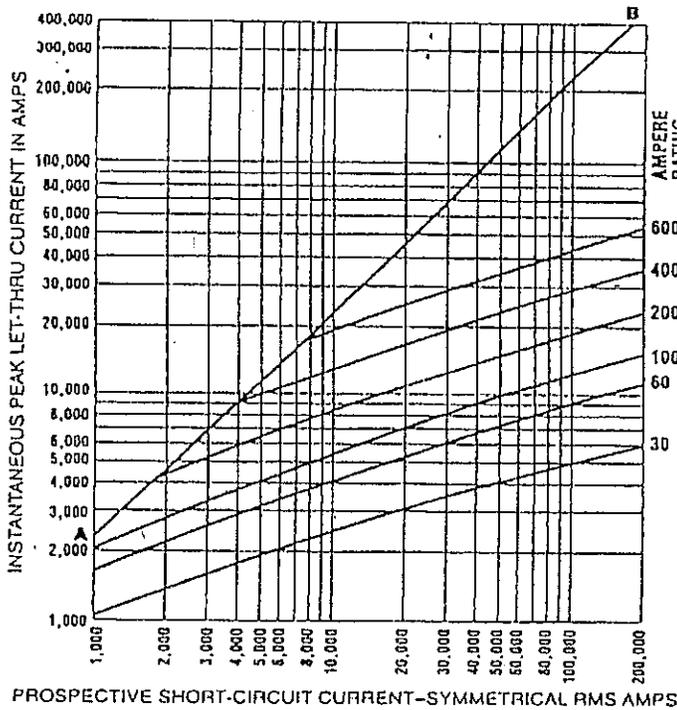
Figure 5.11 Typical Class J peak let-through current data at 600 V. (Cooper-Bussman)
