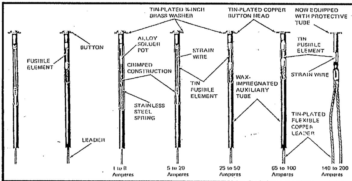
Typical construction of use links – Universal button head fuse links rated 1 through 200
